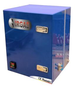
These type of approaches to combustion analysis are not required on the IRGAS FieldView. Its high sensitivity allows the use of a short path gas cell while offering the same sensitivity as other systems using a long path gas cell. For this reason, the analyzer does not require the sample to be dried out, and the flow rates to achieve a fast T90 are under 1 slpm.
