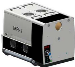
Figure 2: MR-i instrument: 1) MR-i Spectroradiometer, 2) Camera/detector module A, 3) Camera/detector module B, 4) Input telescope, 5) Radiometric calibration sources
